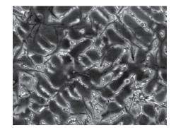
**Fig. 1** Type A graphite in an austenitic matrix with chrome carbide (100x, etched in 5% Nitol)
